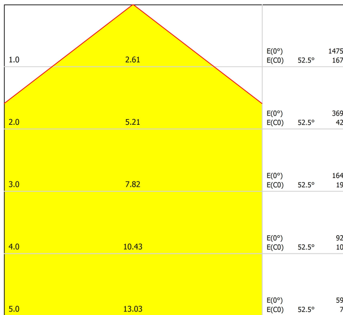
Distance [m] Cone Diameter [m] Illuminance [lx] — C0 - C180 (Half-value Angle: 105.0°)
